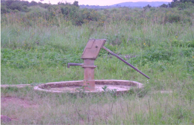
Figure 3: A non-functioning hand pump in Nankoma Town in Bugiri District abandoned in a bushy area
